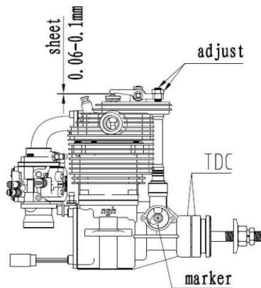
Valve clearance adjustment diagram
