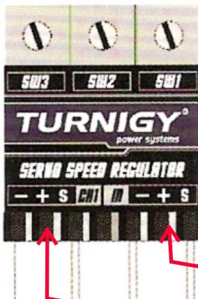
The TURNIGY Slow-down unit is a fully adjustable 3 channel-out device which can be used on any receiver channel and will decrease the servo travel time.
